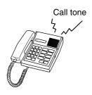
**Step 2.** Lifting the handset stops the call tone and permits conversation to proceed. (A response can also be made by pressing the [PTT] key for handsfree conversation.)
